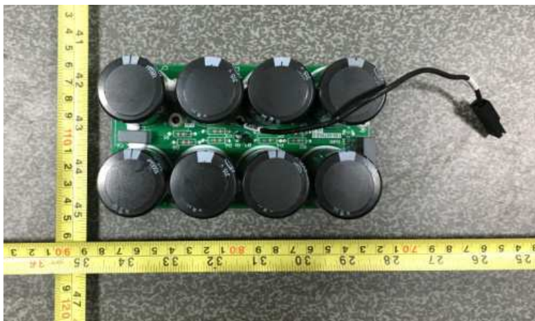
Front view of capacitor board of HYD 4600-EP, HYD 5000-EP, HYD 5500-EP, HYD 6000-EP
